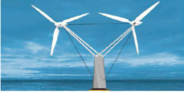
Fig. 1. SEREO structure [Herskovits et al. (2014)] composed of twin wind turbines.
